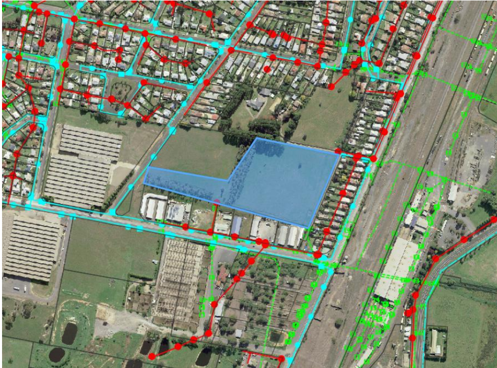
Figure 19. Extract of Council’s mapping showing existing sewer (red), stormwater (green) and water (blue) infrastructure
